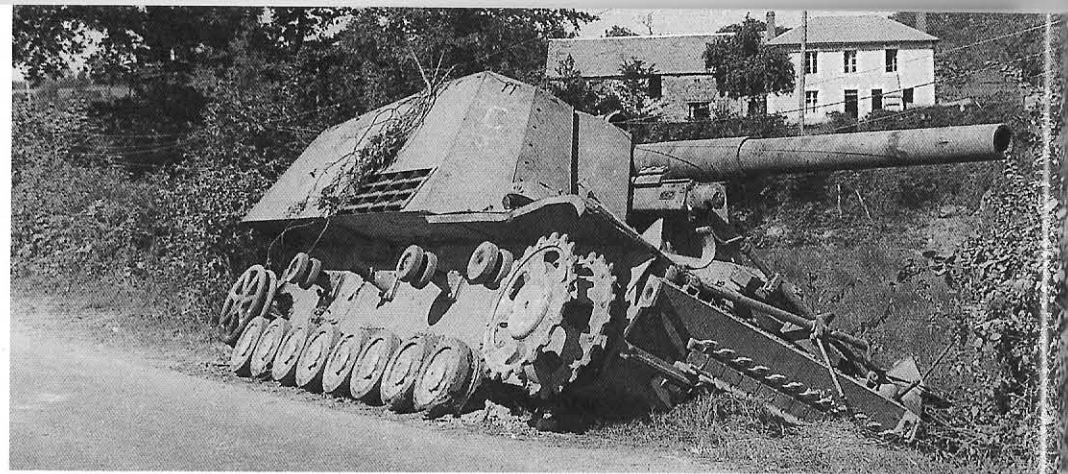
Normandy, late 1944. Note the characteristic bocage of the French countryside. Pushed aside in the wake of the allied advance, this early model vehicle is missing the entire right track and a rubber return roller, probably lost at the same time.
