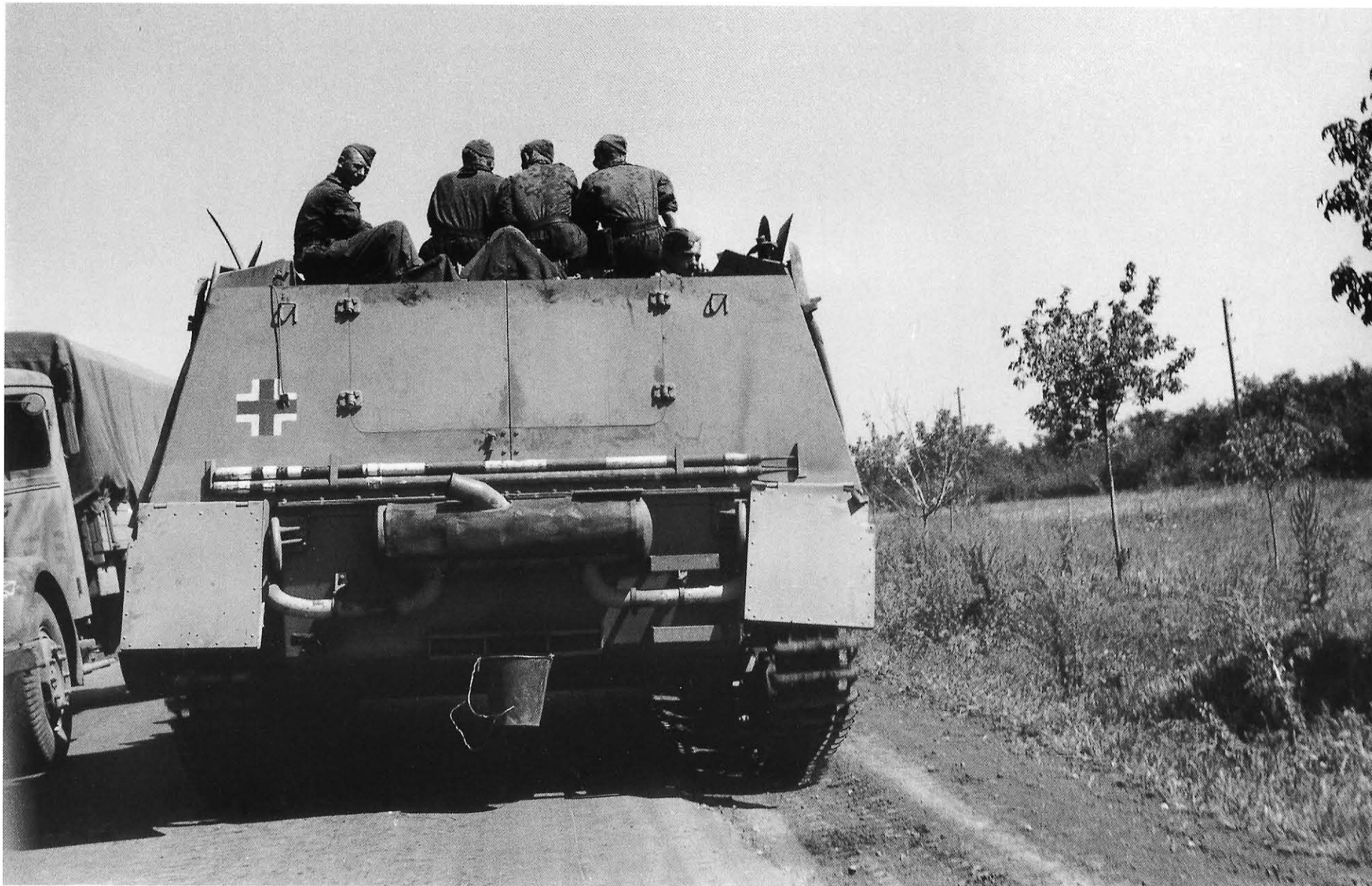
This vehicle from the same unit still retains the large mudflaps behind the rear tracks. These were often lost in hard maneuvering. Note the early version muffler, and the pea-pattern camouflage uniforms of the SS-men. The Balkenkreuz is in its typical location.
