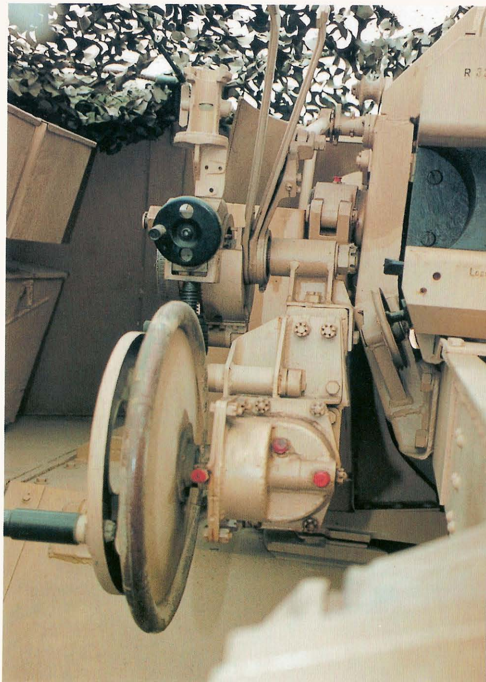
The restored Hummel at Panzermuseum Munster is missing the Rblf 36. The arms jutting upward to the right of the sight housing are the telescopic mount reference pointers. The smaller wheel above the traverse wheel in the foreground adjusted the height of the sights. These elements comprised the Zieleinrichtung 34 aiming sight.
