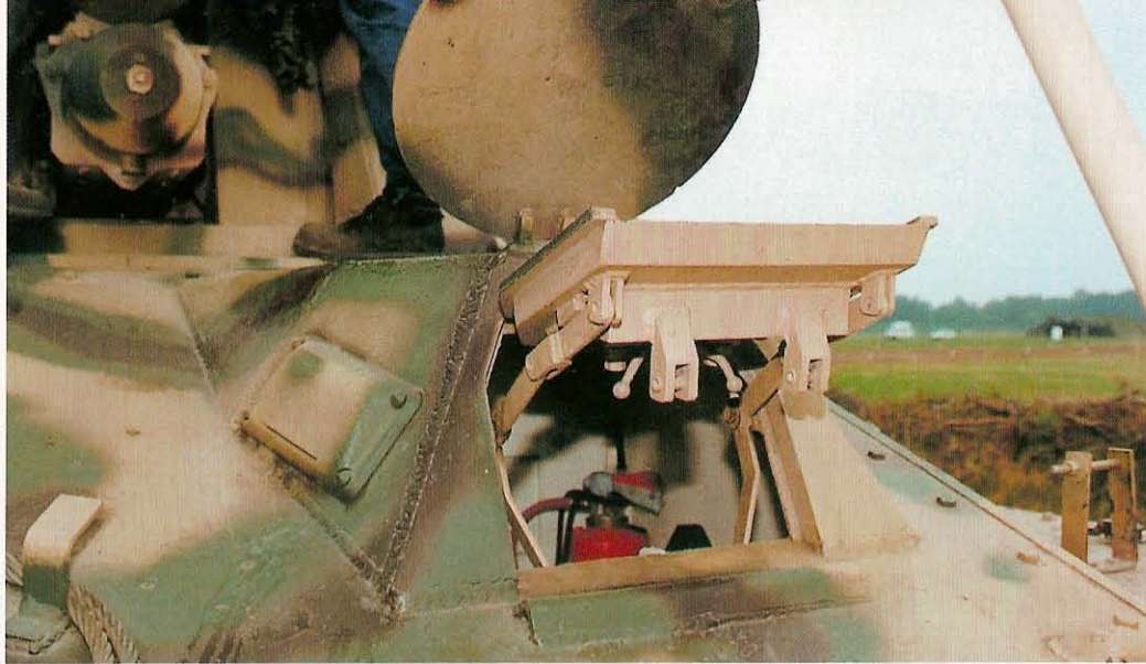
The early version 15cm Panzerhaubitze 18 at the Panzermuseum Munster, North Germany. This view into the driver's compartment shows the fire extinguisher and front vision port mechanism in the open position. The downward pointing brackets held a block of thick glass, now missing.
