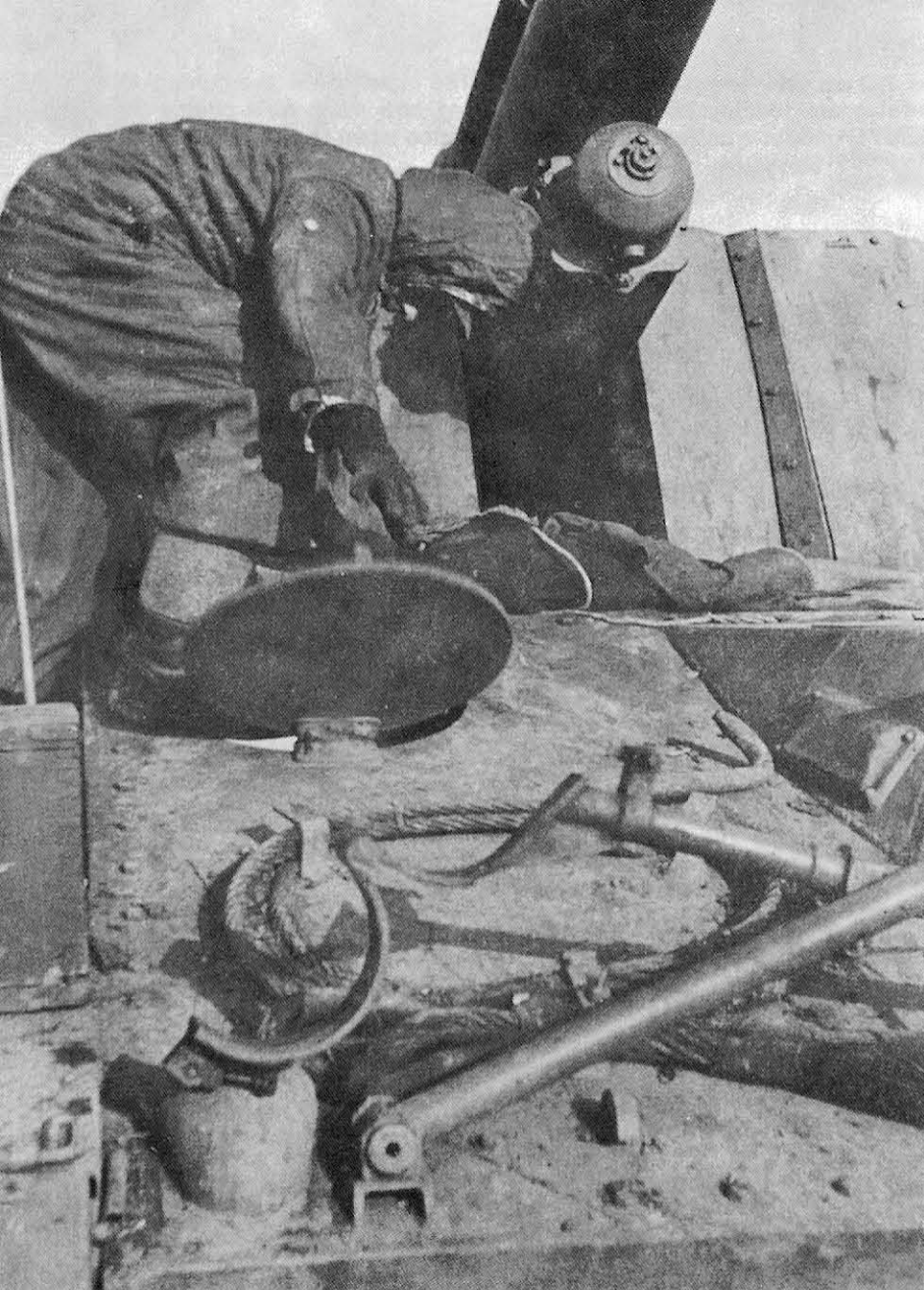
A parka-clad radioman stows his personal gear on his side of the driving compartment of this Hummel. The folded travel lock for the gun barrel is seen in the foreground of the photo.
