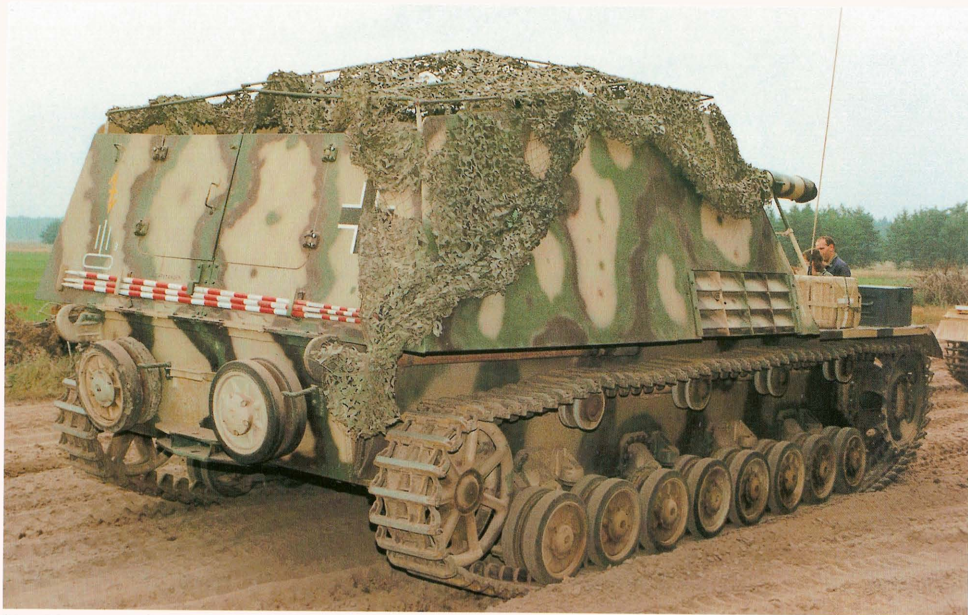
"Anton" bears a camouflage scheme that matches as closely as possible the three original colors available for use: basic dunkelgelb, or yellow tan, green RAL6013 and brown RAL8017. The pipe framework over the crew compartment may remain from the wartime vehicle as part of an anti-grenade barrier. It does not, however, appear to be original.
