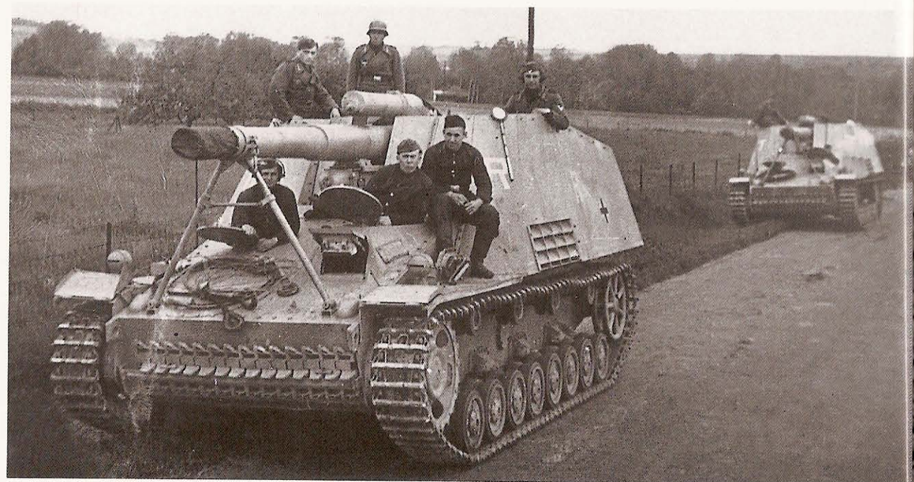
The Ostkette (winter tracks) allowed better mobility over soft terrain through decreased ground pressure. Eastern Front, Russia, January 1944.
