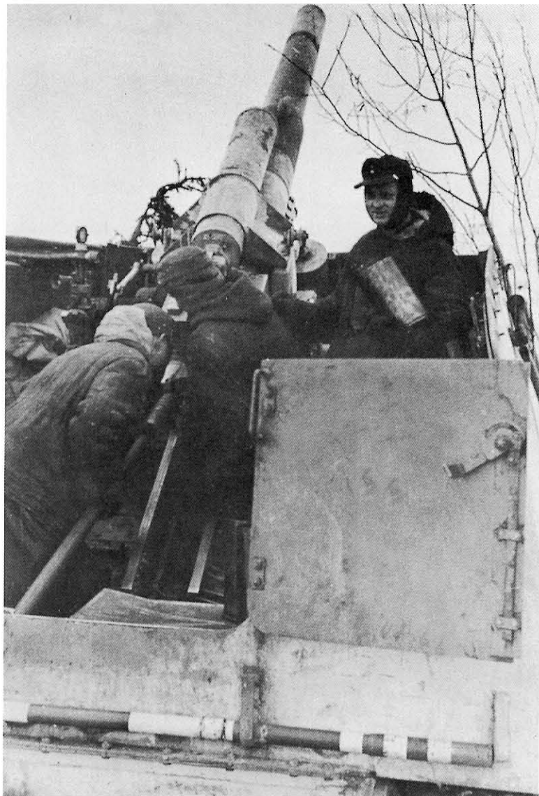
Russia, winter 1944-45. A coat of whitewash blends this vehicle into the landscape. The Balkenkreuz was preserved. As the vehicle only carried 18 rounds, Munitionsträger Hummel would deposit ammunition beside the vehicle during sustained fire engagements.
