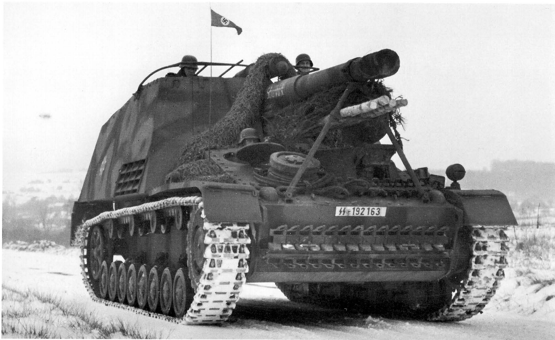
"Scharnhorst" of the same unit. In addition to the spares on the rear hull, a third road wheel seen here was attached to the glacis plate inside the towing cable. The wood beams resting on the cross brace of the barrel support were used as poles to support the camouflage net. The license was painted directly onto the hull of the vehicle, and the swastika pennant was more patriotic than an identification symbol.
