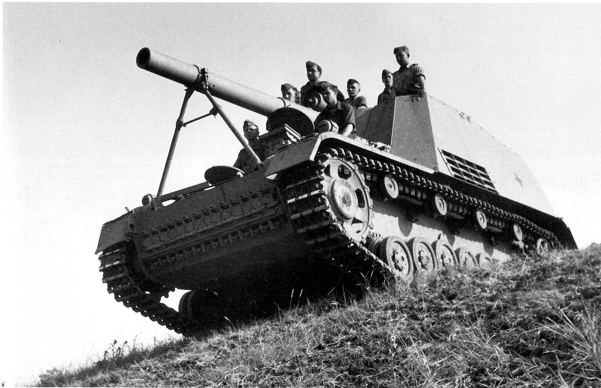
A proud Hummel crew poses with their vehicle. Mobilized artillery was very popular with the ground troops that saw less of their fire support coming from the Luftwaffe as the war continued. Note the spare track that was typically mounted at the front of the hull, and the rubber rimmed return rollers. Each crewmember had a steel helmet in addition to the field caps worn here.
