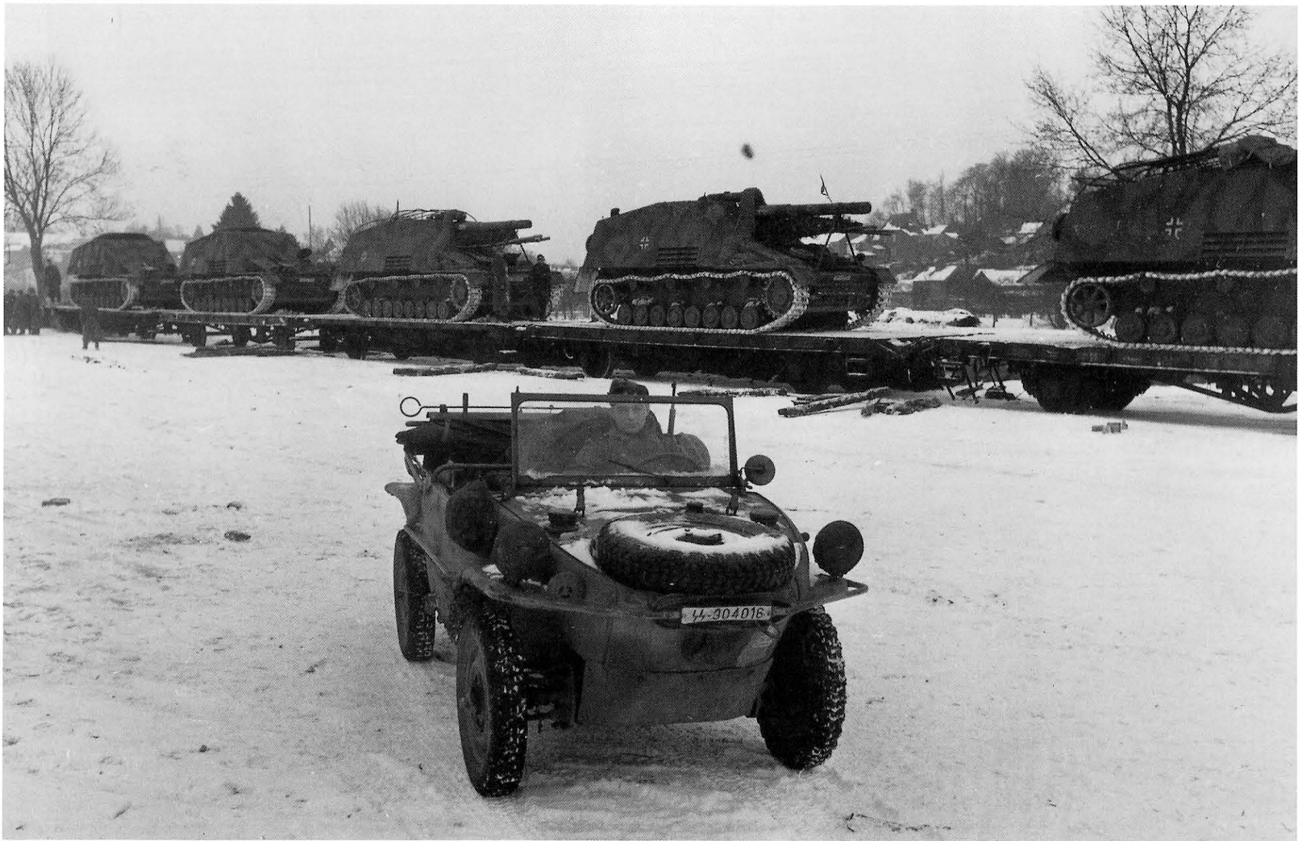
This Volkswagen type 166 “Schwimmwagen” (Kfz. 1/20) of the artillery battery features a tactical sign with the letter “s”, meaning “schwere” (heavy). The last two vehicles are Munitionsträger Hummel. These brand new vehicles would be additionally modified after arrival with appropriate snow camouflage.
