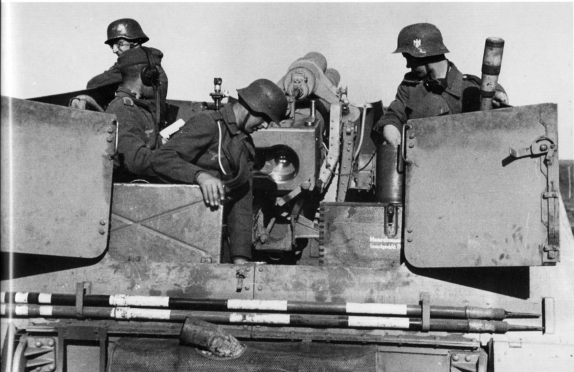
Hummel crew in action. The gun commander receives plotting coordinates, one Kanonier handles the rounds and another is ready to position the rounds in the barrel. The red and white ranging rods are clearly seen in their holders.
