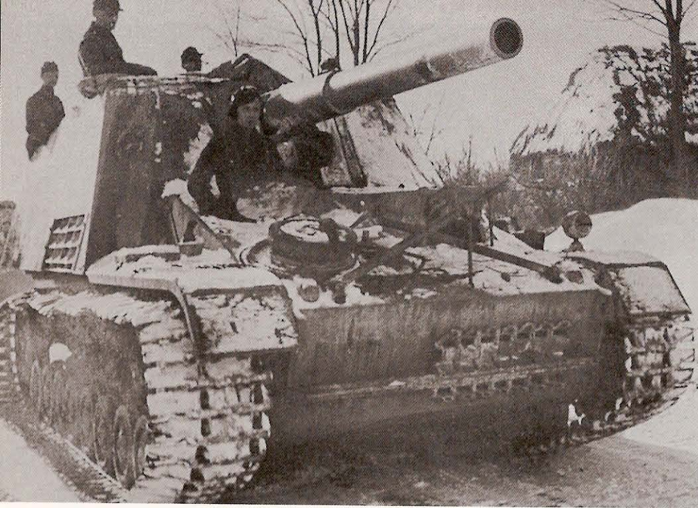
The Ostkette (winter tracks) allowed better mobility over soft terrain through decreased ground pressure. Eastern Front, Russia, January 1944.
