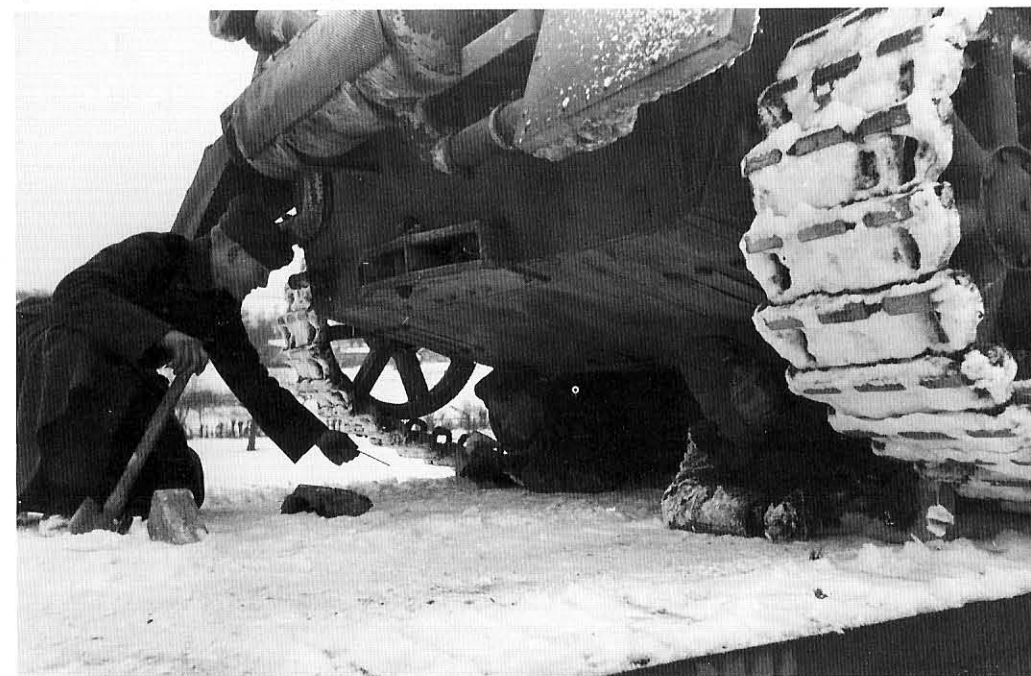
The Fahrer (driver) of Panzerhaubitze "Blücher" is carefully guided off the platform. These two axle flatcar wagons are of standard gauge width (1435mm), as this gauge was used throughout Europe with the exception of Spain. The Soviet Union employed the wide gauge (1528mm) rail tracks, a significant challenge to German logistics.
