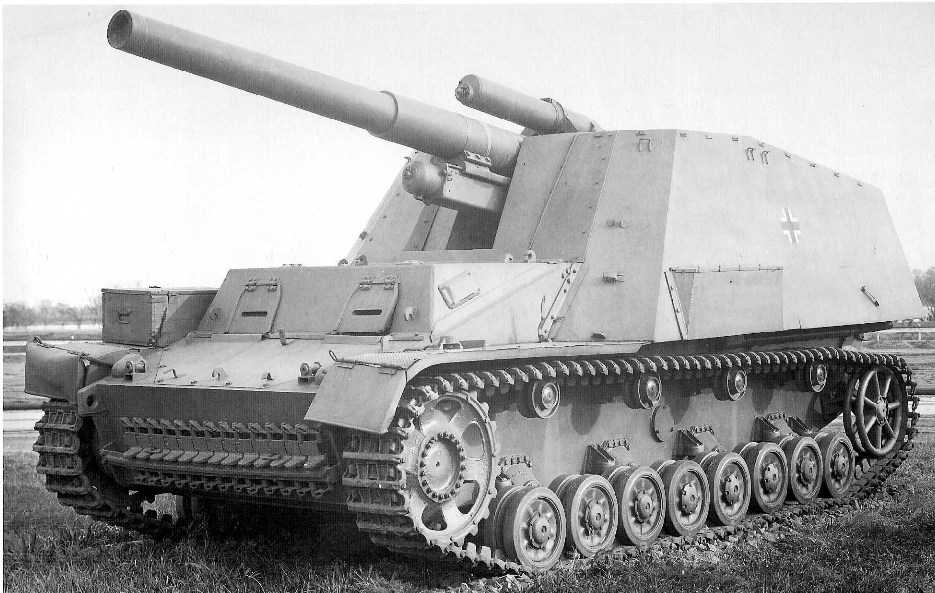
This late model vehicle has a thin plate of armor over the engine air intake louvers. It is missing its headlight, as this version carried only one Bosch headlight on the left treadplate fender. Shadow gives good definition to the circular plate cover of the preheating system for the cooling water, located in the middle of the lower hull.
