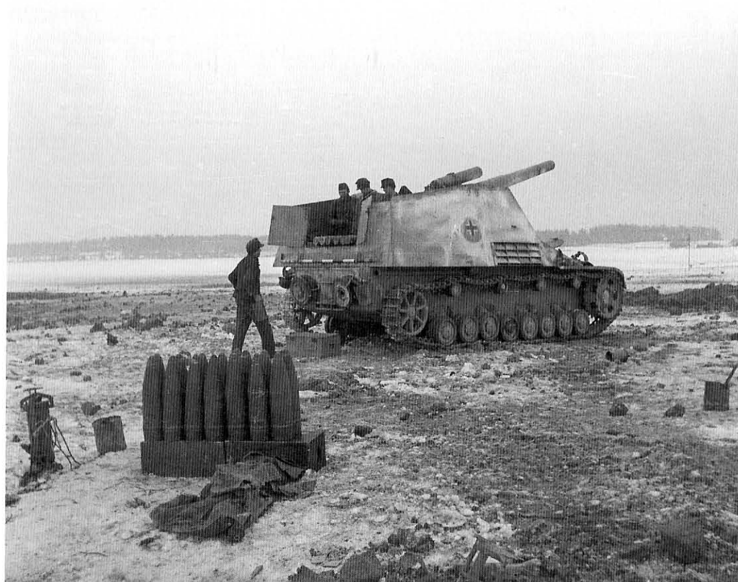
Russia, winter 1944-45. A coat of whitewash blends this vehicle into the landscape. The Balkenkreuz was preserved. As the vehicle only carried 18 rounds, Munitionsträger Hummel would deposit ammunition beside the vehicle during sustained fire engagements.
