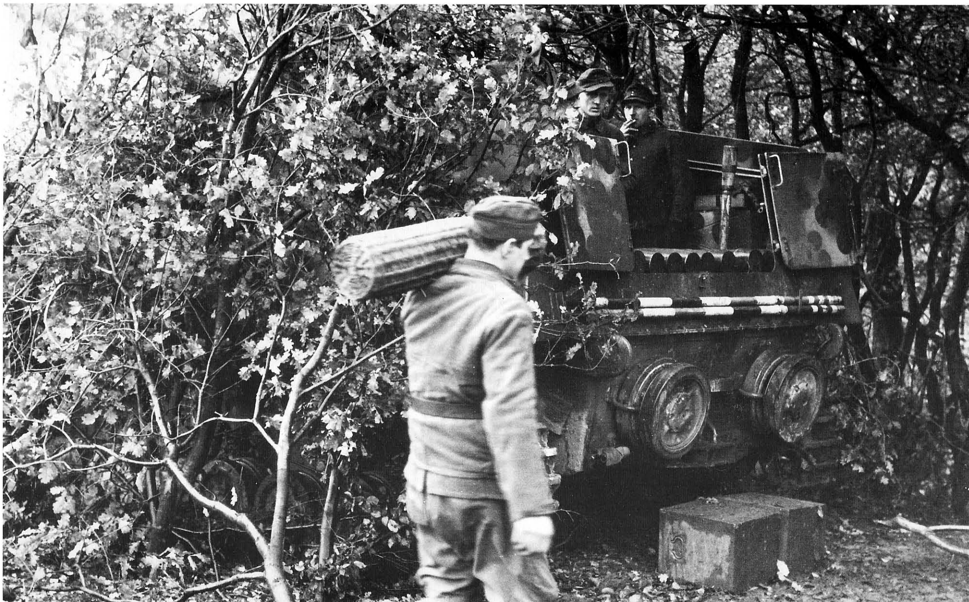
Wicker baskets protected the rounds from the jostling effects of transport. This late model vehicle is preparing for sustained fire, given the ready rounds stacked at the hull rear on top of the internal shell cabinets. Note the tri-color paint scheme evidenced on the right rear door. Late war German vehicles bearing camouflage on interior surfaces testify of an anxiety to avoid detection.
