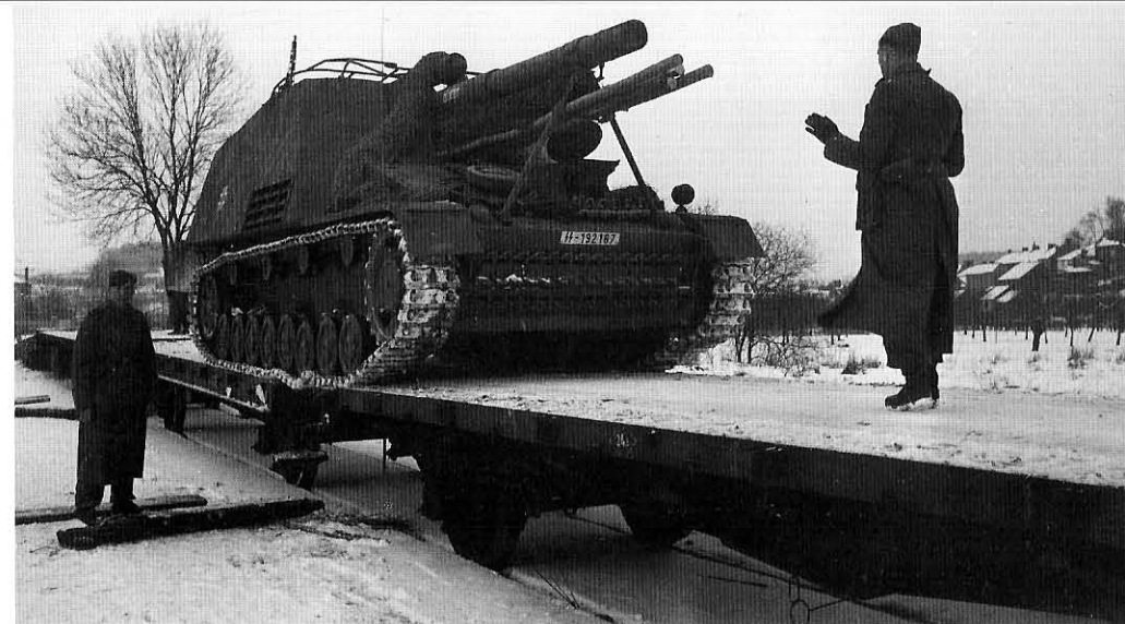
The Fahrer (driver) of Panzerhaubitze "Blücher" is carefully guided off the platform. These two axle flatcar wagons are of standard gauge width (1435mm), as this gauge was used throughout Europe with the exception of Spain. The Soviet Union employed the wide gauge (1528mm) rail tracks, a significant challenge to German logistics.
