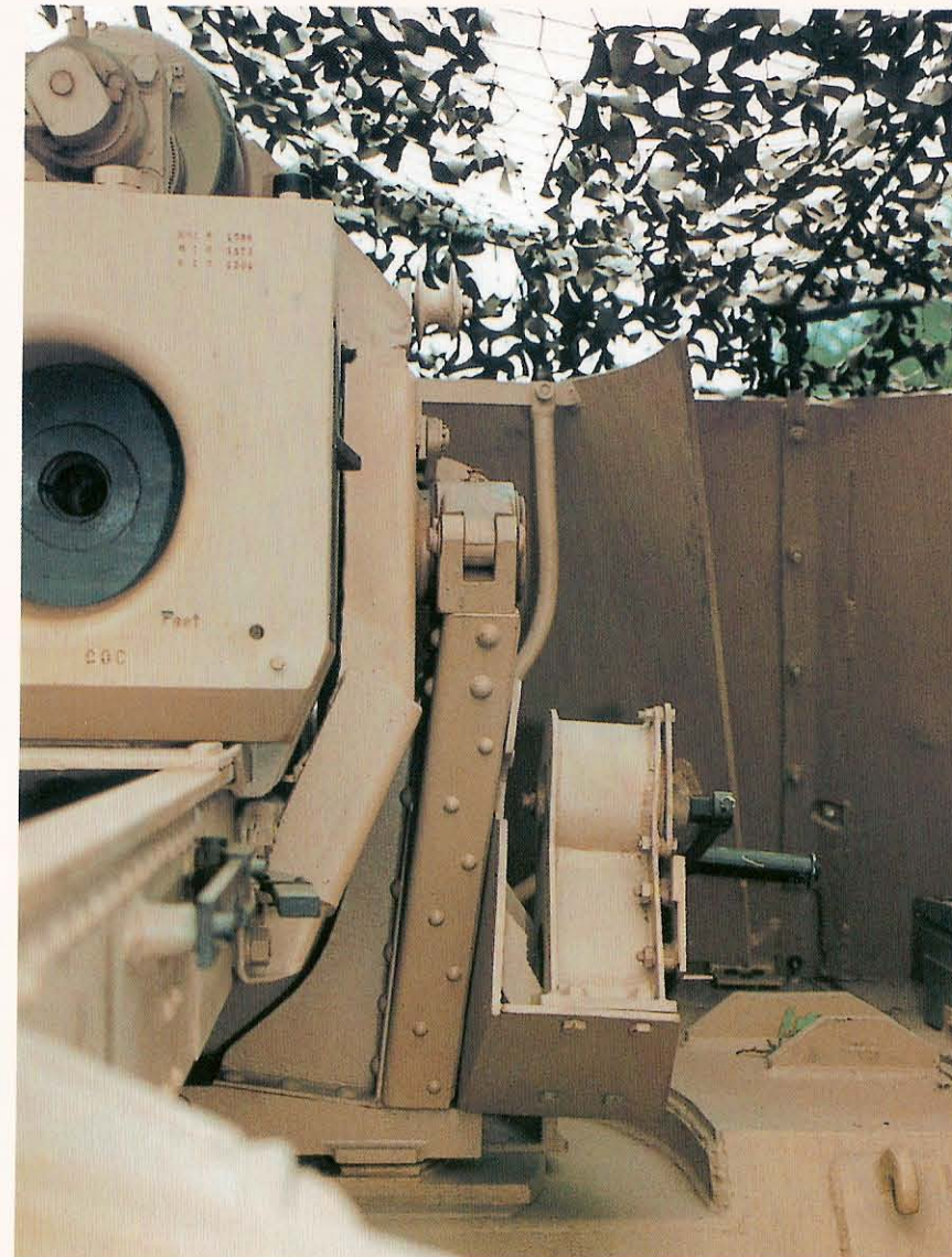
The restored Hummel at Panzermuseum Munster is missing the Rblf 36. The arms jutting upward to the right of the sight housing are the telescopic mount reference pointers. The smaller wheel above the traverse wheel in the foreground adjusted the height of the sights. These elements comprised the Zieleinrichtung 34 aiming sight.
