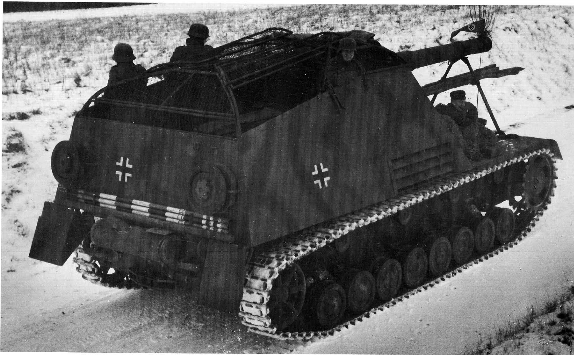
Polish Galicia, October 1943, during railroad unloading. The 9. SS-Pz. Div. "Hohenstaufen" made significant field modifications to their Hummel, and attached one spare road wheel to either side of the access doors. These vehicles are of the Pz.Ar.Rg. 1. The screens over the fighting compartment protected the crew from grenades and inclement weather, as tarps were drawn over the framework.
