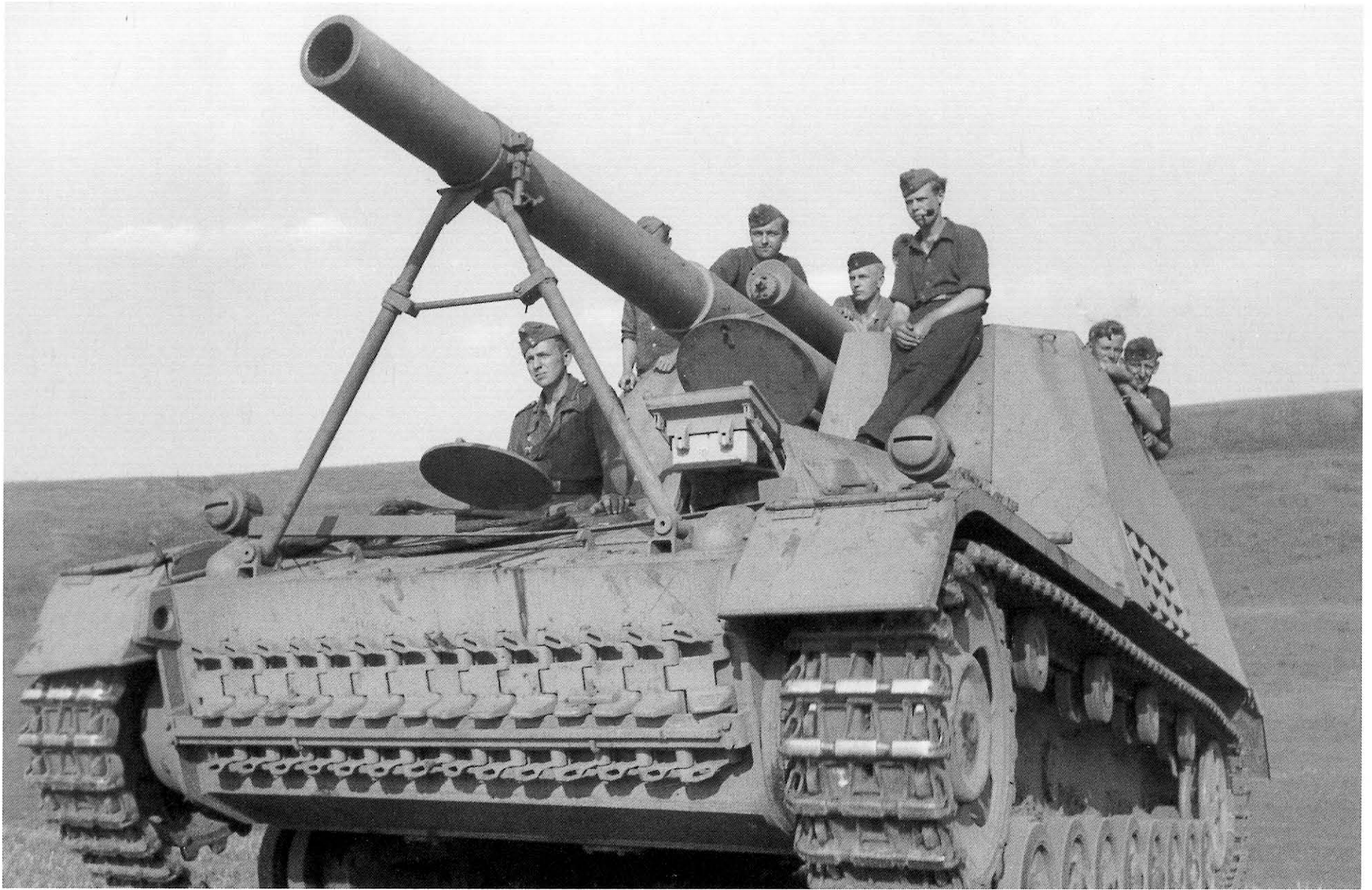
Russia, 1943. This Hummel crew pauses well behind the front lines for snapshots. The gun travel clamp was unfolded from the hull and attached manually to the barrel. The strut between the arms was always affixed to the left support, and pivoted into position to steady the frame.
