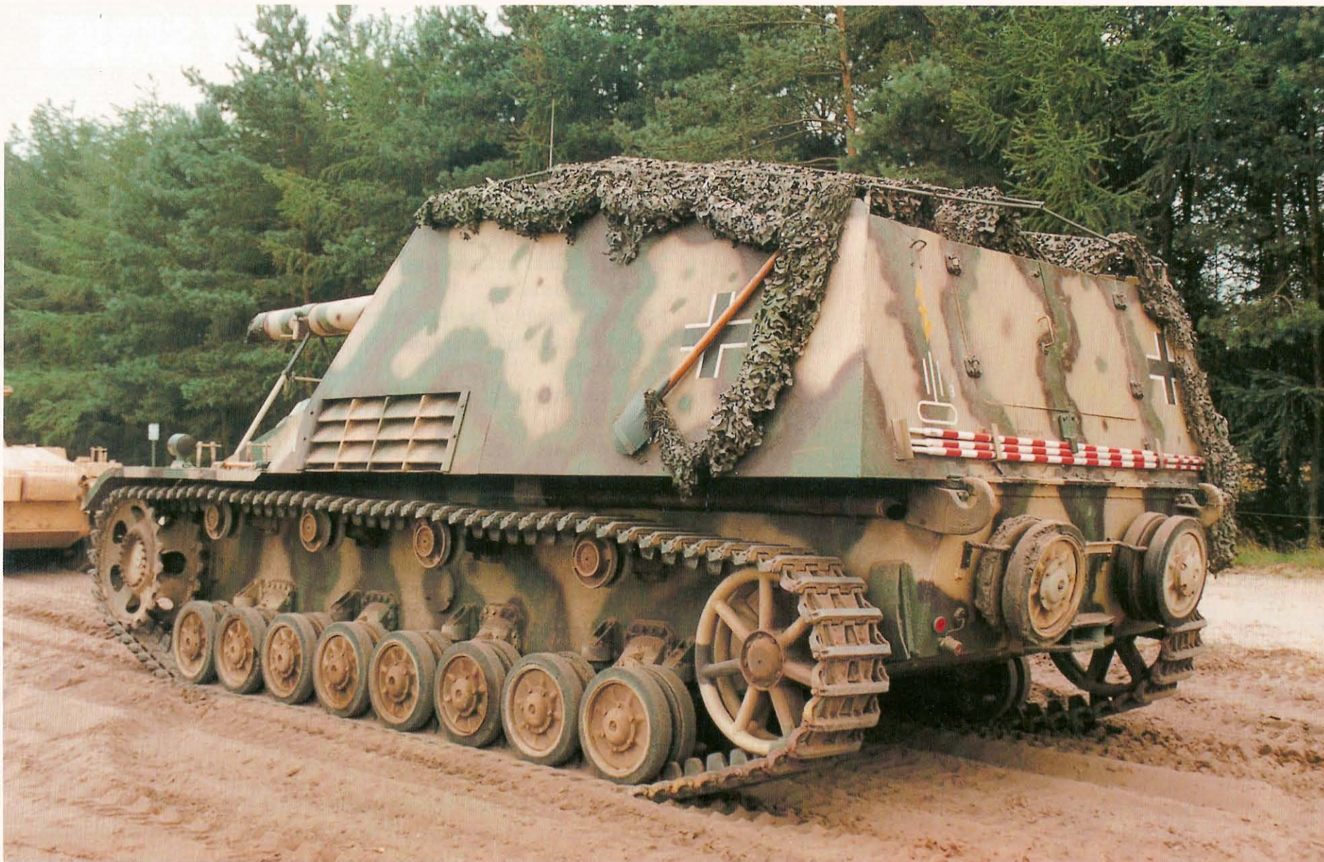
Restored "Anton" sports modern-style camouflage netting, though the practice of using netting was common in the history of the vehicle. This view shows the later spare road wheel configuration on the lower hull rear. Note the Balkenkreuz and the tactical sign representing a fully tracked artillery piece.
