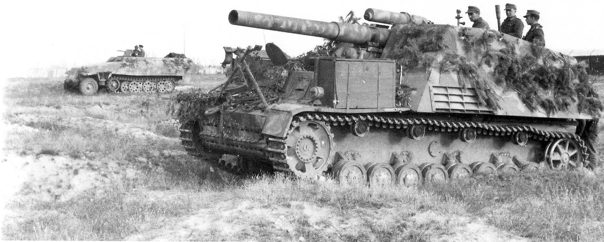
Eastern Front, 1944. This late model vehicle carries an effective combination of hand-applied paint and vegetation. A custom box carries rounds for the s.FH. 18, given the visible load exerted on the fender. Shell weight ranged from 25 Kg. for the AP and 45 Kg. for the HE ammunition.
