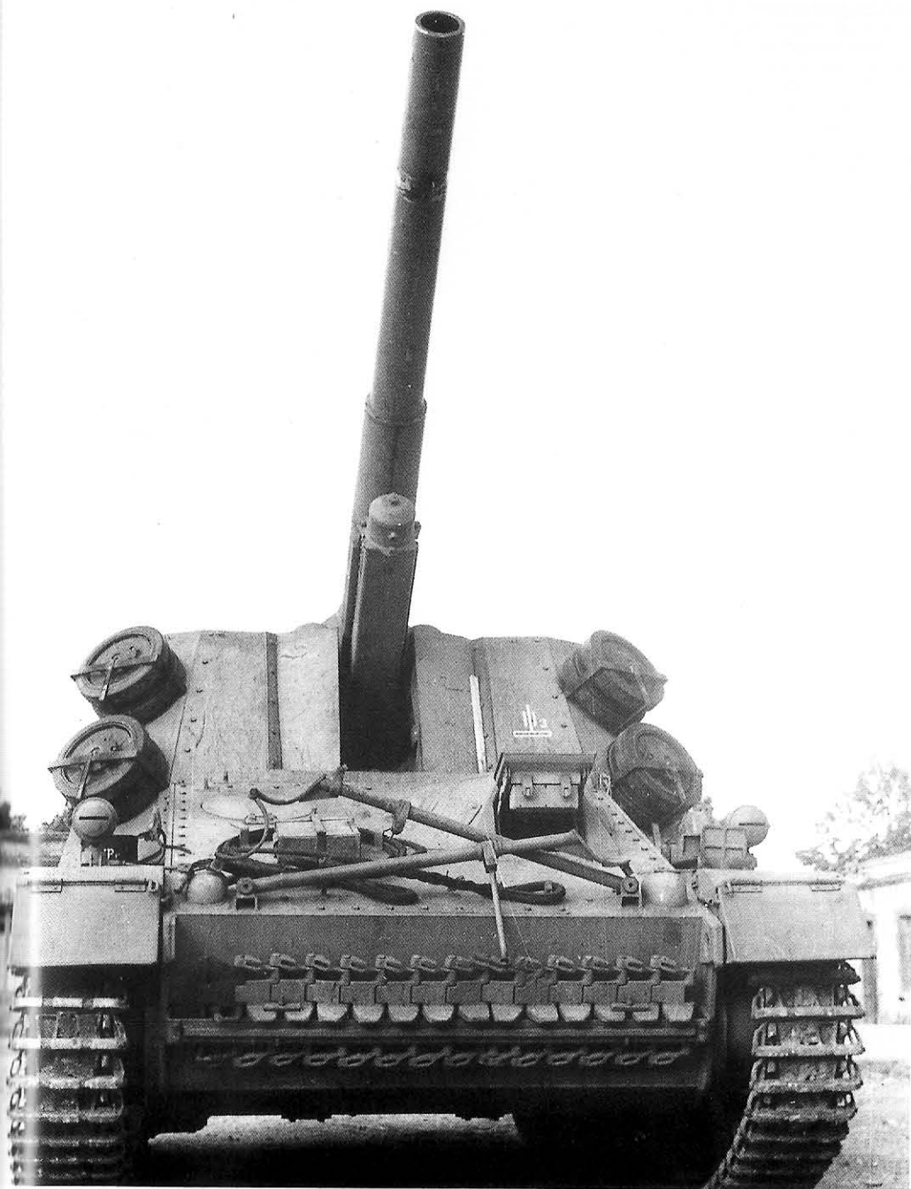
A crewman disengages the foldable gun travel clamp. The tow cable lays at his feet. Note the thick glass block under the open visor that protected the driver. The mudflap in the foreground was pinned in place and spring-assisted. These were often lost in cross-country conditions.
