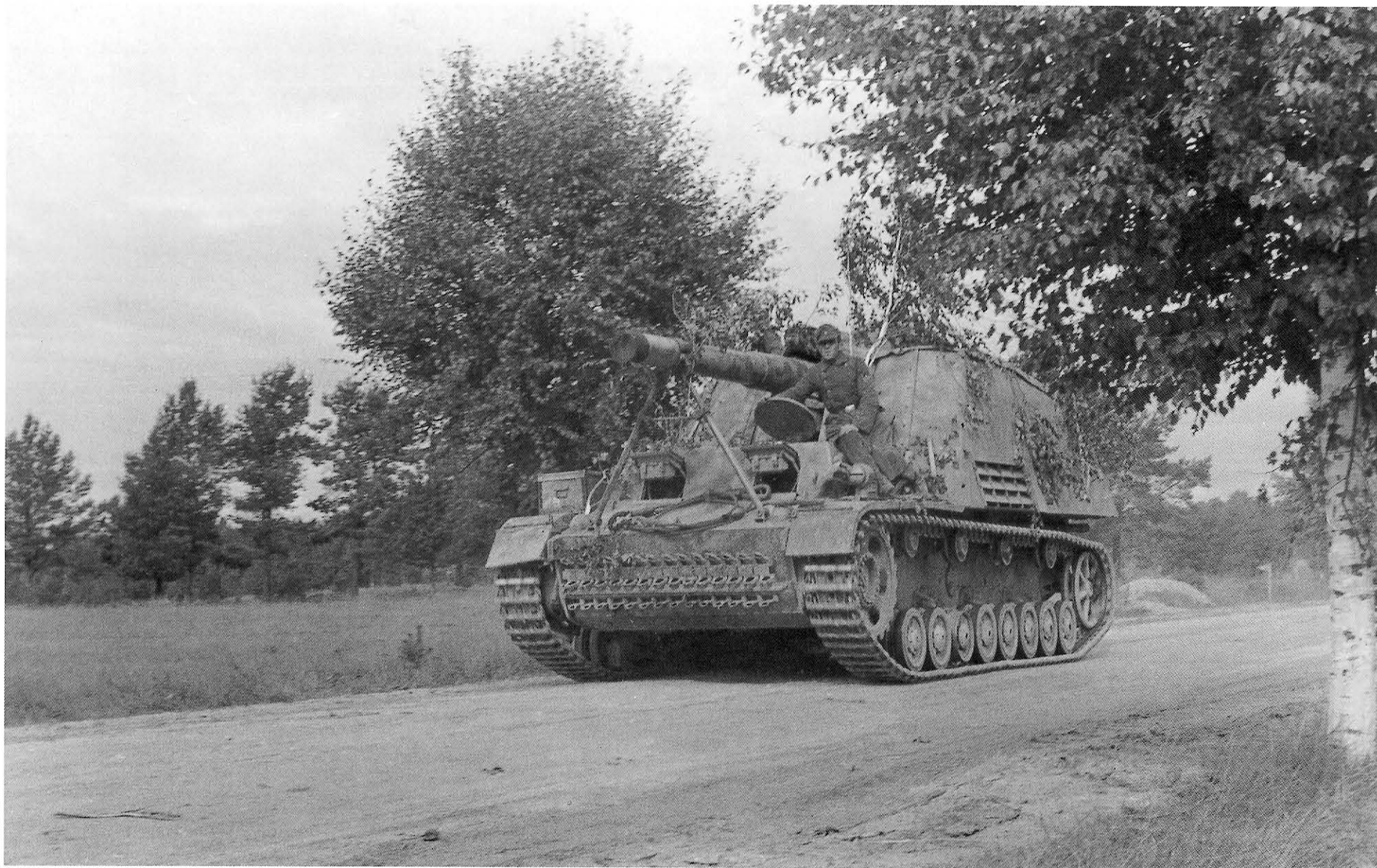
This late model vehicle in Normandy features the full compartment added for the radio operator's comfort and visibility. This change was made in early 1944. Allied air superiority and defensive operations dictated that German vehicle crews take measures to conceal their equipment. This vehicle sports a heavy mottling of airbrushed camouflage, along with branches to break up its silhouette.
