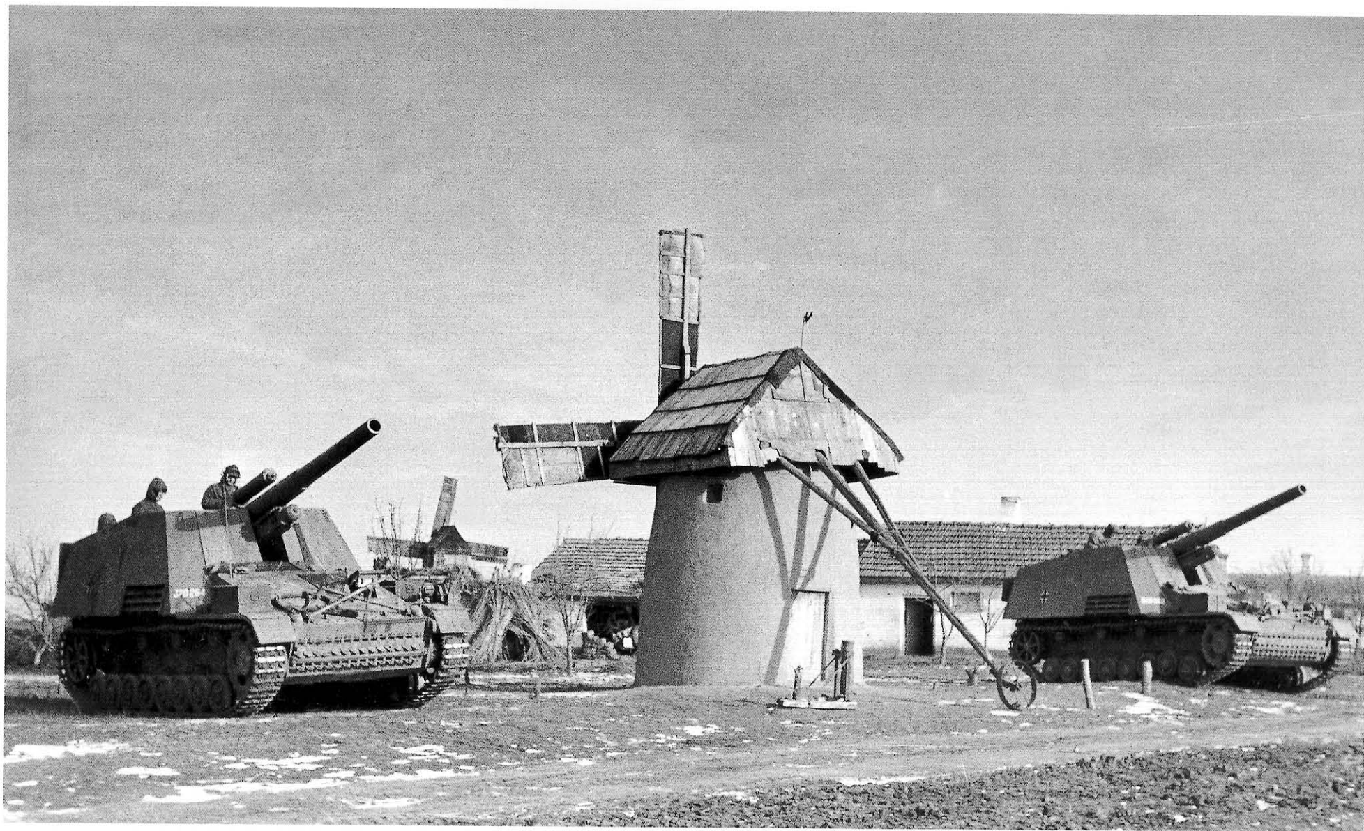
Russia, Spring 1944. These Hummel of the 1. Panzer Division carry custom-made rectangular frames welded to the right of the lower hull, which helped the driver move into firing position. Planners specified an all-round fire capability, but accepted the forward-fixed arrangement. Extemporized tools such as the driver's sighting frames went some distance toward enhancing the rapid deployment of the howitzer.
