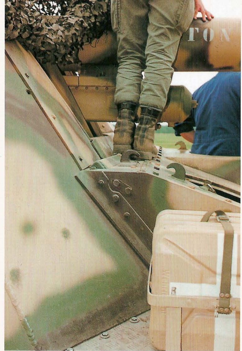
The downturned hooks on the top of the hull crew compartment allowed the armor plate to be lifted in case of repairs. The treadplate of the fender in the lowest portion of the photo is not an original pattern.
