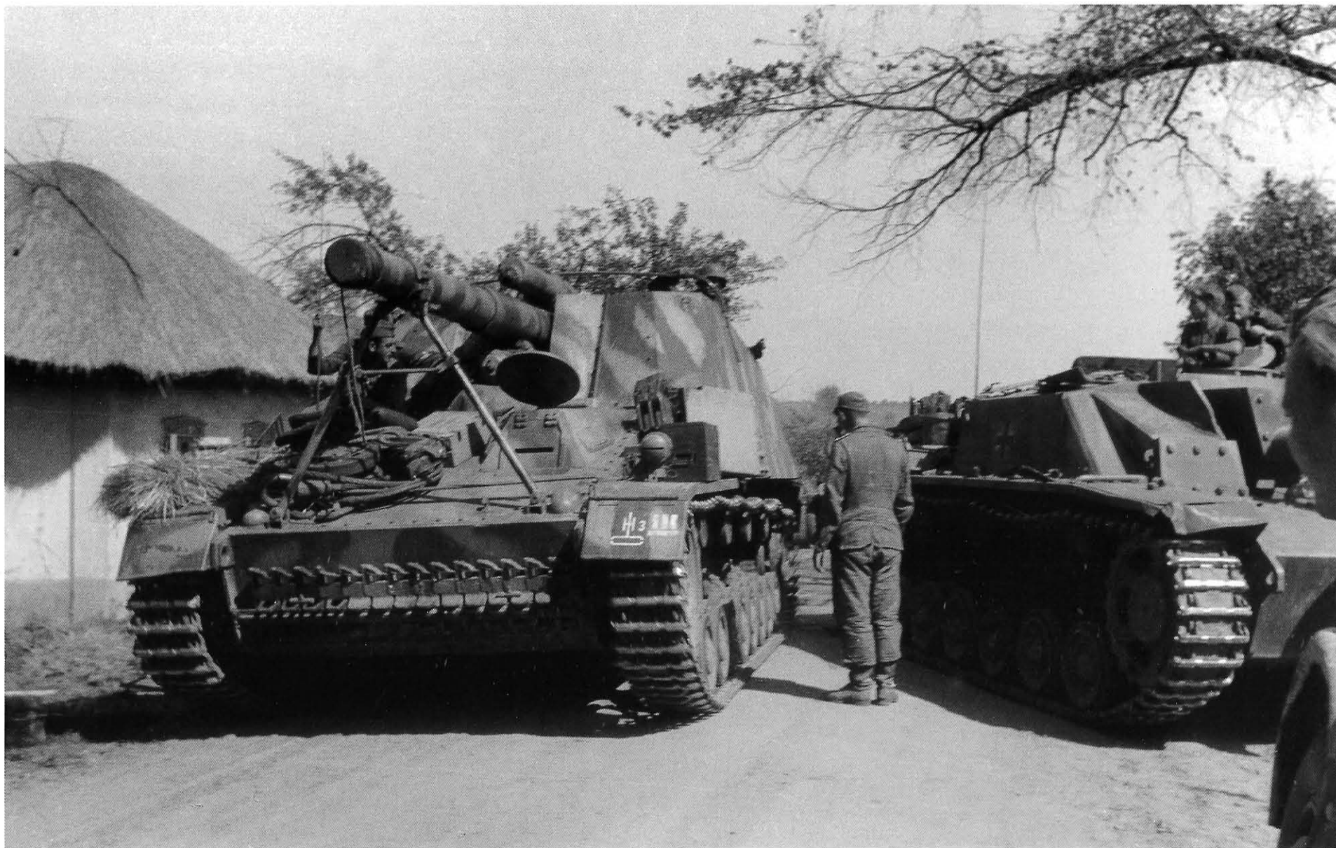
Russia, 1943. This early version vehicle sports an elaborate field applied camouflage scheme. Note the tactical sign on the fender, the tow cables on the glacis plate, and the combination of solid and hollow guide-horn spare track links.
