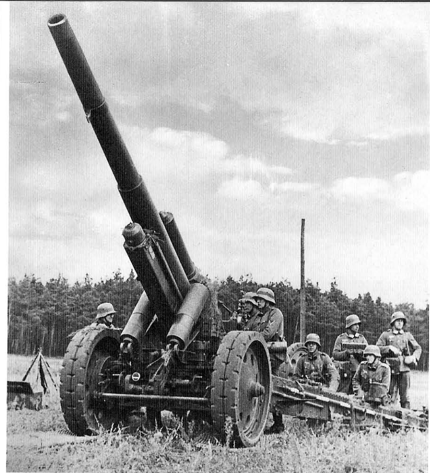
The 15 cm schwere Feldhaubitze 18L/29.6 was developed and built between 1926 and 1930 by Krupp and Rheinmetall. The howitzer had a maximum range of 13,325 m and a rate of fire of 4 rds. per minute.
