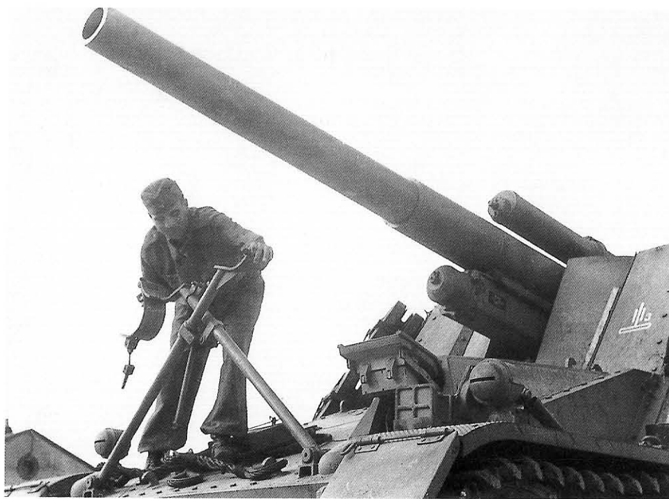
A crewman disengages the foldable gun travel clamp. The tow cable lays at his feet. Note the thick glass block under the open visor that protected the driver. The mudflap in the foreground was pinned in place and spring-assisted. These were often lost in cross-country conditions.
