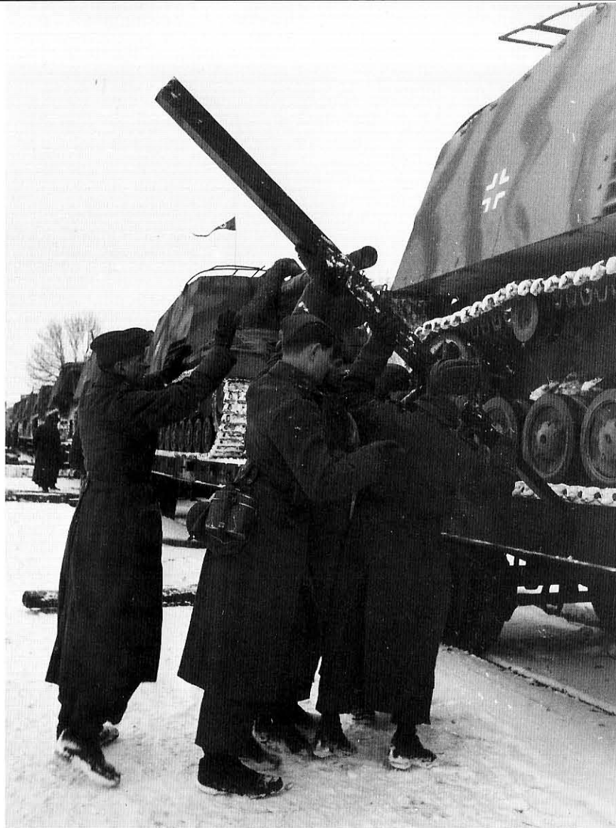
The Hummel are prepared for unloading. Crewmen pry apart the track from the frozen surface of the flatcar. Note the hollow guide horns of the earlier type track links.
